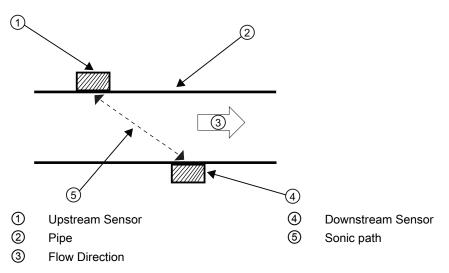
Figure 5-3 Direct Mount (Pipe shown from above in 12 o'clock position)
