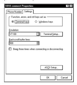
8. Next, left-click on the [ASCII Setup] button (see screen above). In the [ASCII Sending] dialog box, make sure that both [send line ends with line feeds] and [Echo Typed characters locally] are UNCHECKED. In the [ASCII Receiving] dialog box, left-click to place a check mark before the [Append line feeds to incoming line ends] dialog. When your screen looks like the example below, left-click the [OK] button.
