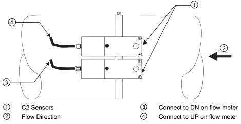
Figure 7-2 Adjacent Sensor Mounting
