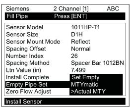
5. Refill the pipe completely, then press <ENTER>.
