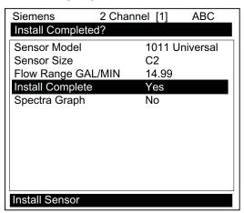
The flow meter is now operational and the display will show flow by pressing the <MENU> key.
