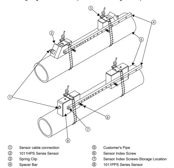
Figure 5-10 Reflect Mount with EZ-Clamp and Spacer Bar
