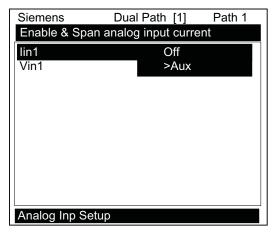
2. Move the cursor down to [Aux] by pressing the <Down Arrow> and then press <ENTER>. This enables the port to receive an input current. The cursor moves to [4 mA].
