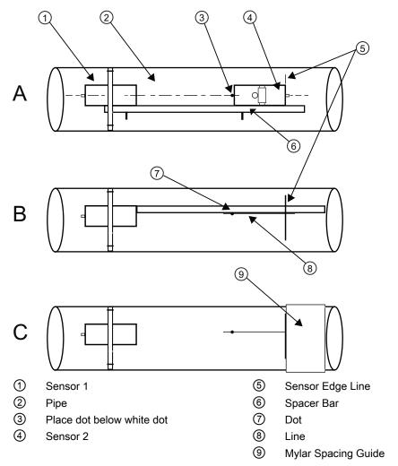
16. Wrap the Mylar spacing guide around the pipe so that the left edge is against the sensor edge mark (see "C" above). Arrange so that one end overlaps the other by at least 8 cm (3 inches). Trim to fit if necessary, but in order to keep the end square, be sure not to trim at the overlapping end.
