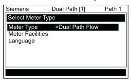
4. Press <ENTER> to select. Press <Right Arrow> to select meter function. Press <ENTER>.
