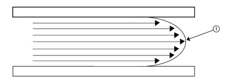
1 Fluid velocity near the axis of the flow stream tends to be greater.
