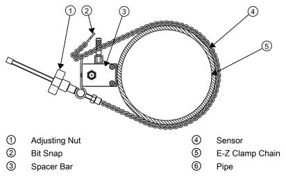
Figure 5-11 Sensor Mounting with E-Z Clamp and Spacer Bar
