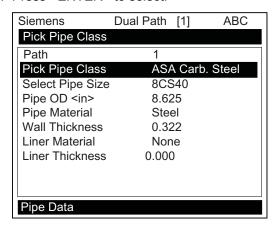
4. Pre-programmed Pipe Size and relevant pipe parameters will appear in menu cells. Press <Right Arrow> and scroll to desired pipe size. Press <ENTER>. Enter dimensions manually if pre-programmed dimensions do not match application.
