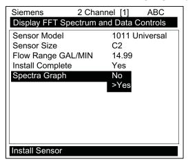
The Spectra Graph display shows the results of the Fast Fourier Transform (FFT) performed by the flow meter.
