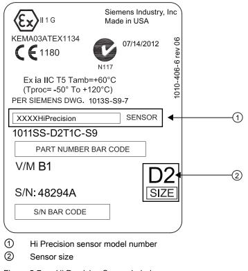
Figure 5-7 Hi Precision Sensor Label
